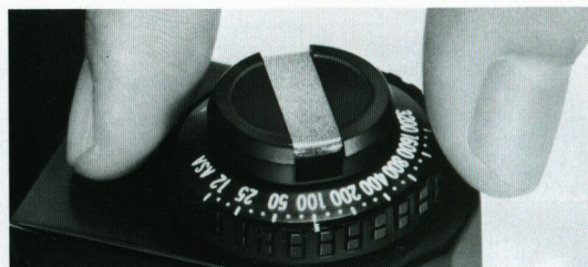
ASA film speed ring and exposure compensation dial coaxially located around the film rewind crank.
