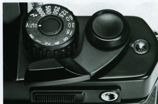
Unique electromagnetic release button on hub of film advance lever. Film advance lever unlocks the exposure check button of full return. Shutter control dial has AUTO setting, as well as full-range manual shutter speed settings from 1 ~ 1000 sec. plus B & flash synch ( \lambda ).
