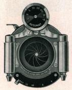
The Automatic is operated by either bulb attachment or finger release. It is a very compact shutter and for exposures of 1,  $\frac{1}{2}$ ,  $\frac{1}{5}$ ,  $\frac{1}{25}$ ,  $\frac{1}{50}$  and  $\frac{1}{100}$  seconds, works with a constant accuracy hitherto unobtainable. An Iris diaphragm is also supplied and the stops are graduated according to the universal system.
