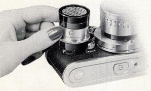
Having mounted the meter on the camera, set the exposure index of your film. This adjusts your meter for the film's sensitivity.
