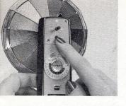
With a flashbulb in place, you can test the entire flash circuit and bulb with the TEST LIGHT button. If everything is working, the white spot above the EJECT LAMP button will flash briefly as the TEST LIGHT button is pressed.
