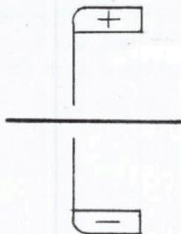
These lenses are provided with the internal diaphragm coupling. After having set the correct ASA film speed and selected a diaphragm opening, press the exposure meter activating button. In the viewfinder the needle will move either in + (over) or - (under) direction. Adjustment can now be made by turning either shutter speed dial or diaphragm ring till the needle reaches the center position.
