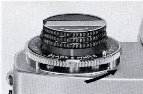
The film memory dial serves also as a release lock for the interchangeable viewfinder system. Turning the dial to the right will release the viewfinder lock.
