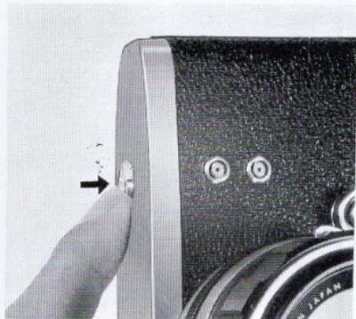
1. First, the film rewind release button on the base of the camera body is pushed in until a small click is heard. This button need not be held during rewinding. The film is now free from the sprocket which has been advancing it, and is ready for rewinding.
