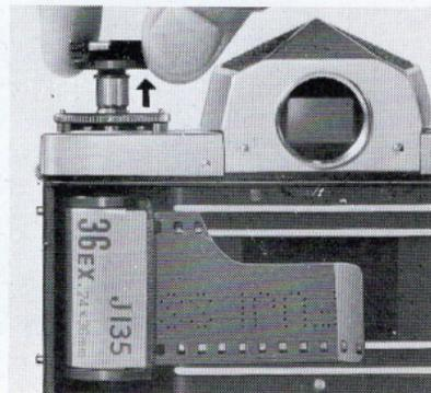
3. Open the back cover by depressing the lock button and pulling up the cover clip at the same time. Pull up the rewind knob and take out the film cartridge. Make certain that no film chips or dust particles are left in the camera.
