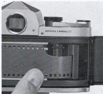
**5. Insert tip of film into spool's film slit**
