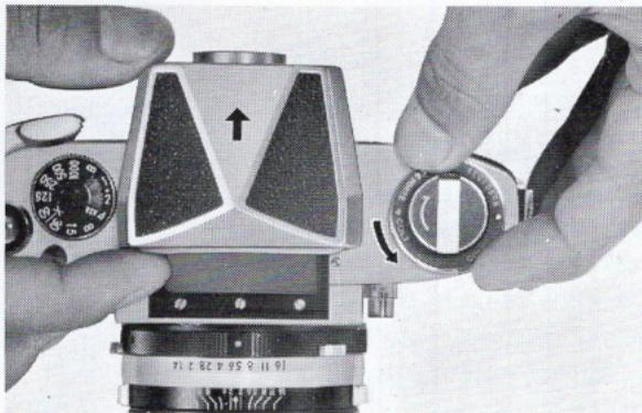
The viewfinder on the MIRANDA Sensomat is interchangeable and can be changed with the most convenient type according to the purpose of the shot so as to make best use of the camera's capacity. The viewfinders available are the pentaprism type and waist-level finders Types VF-1, VF-3 and VF-4.
