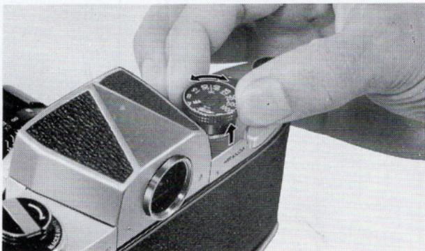
The CdS meter of the MIRANDA Sensomat is coupled to the film speed dial. After loading the film, therefore, see that the film speed dial is set properly. Failure to adjust this dial according to the speed rating of the film loaded in the camera will prevent the meter from giving correct exposure reading.
