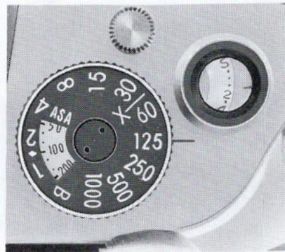
**9. When film counter indicates "1" it means film loading is completed**
