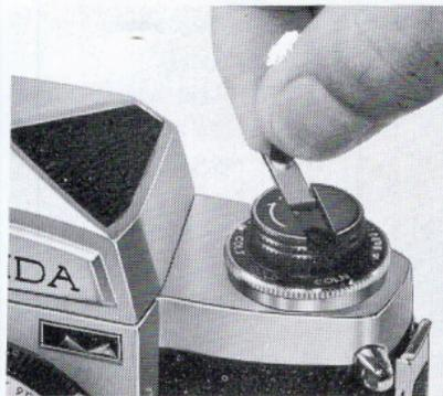
2. Flip the rewind crank on the rewind knob and wind in the direction of the arrow. At the end of the roll you will feel the resistance increase and then suddenly cease. Turn the rewind crank several more times to make certain the film has been entirely rewound.
