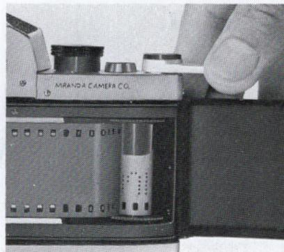
**6. Turn film advance lever until perforations on both sides of film are engaged by the sprocket**
