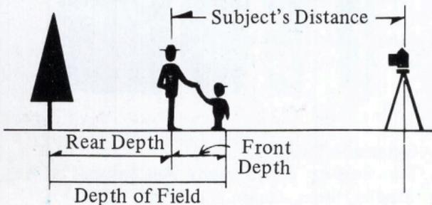
At the center of the lens barrel, facing up, is the depth-of-field scale which indicates the depth of field at a glance. The picture shows the focus adjusted to 2 meters, indicating that the range in which sharp images can be obtained extends from 1.75 to 2.5 meters at  $f/8$  aperture and about 1.5 to 3 meters at  $f/16$ .
