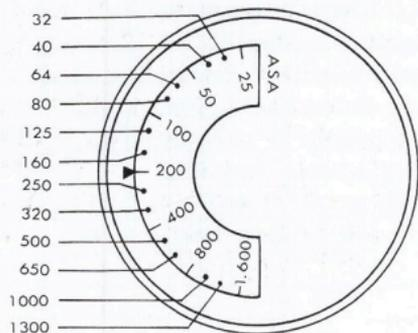
The CdS meter of the MIRANDA Sensomat is coupled to the film speed dial. After loading the film, therefore, see that the film speed dial is set properly. Failure to adjust this dial according to the speed rating of the film loaded in the camera will prevent the meter from giving correct exposure reading.
