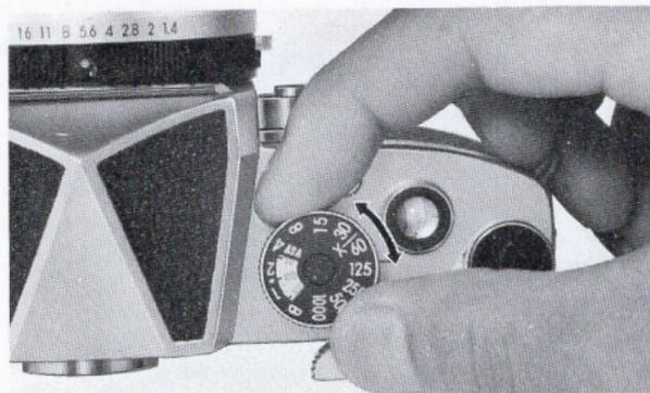
To set the shutter speed, the shutter speed dial is turned to the left or right until the desired speed number lines up with the shutter speed indicator. The dial rotates in either direction.
