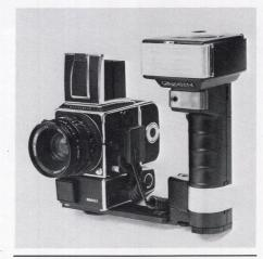
On the Hasselblad ELX the "dedication" is accomplished by means of adapters. Two are presently available, and one or the other will work with various European made flash units. Shown here is the Metz 45 CT-4. The sync cable from the flash unit goes into the adapter mounted on the accessory rail of the camera and the adapter is connected to the six pin socket on the side of the ELX. The film sensitivity is set on the ASA dial on the side of the camera.
