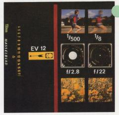
At the same EV value (12 in illustration) you can photograph at a large aperture (f/2.8) (little depth of field) and high shutter speed 1/500 second to freeze the action, or blur the action at a slow speed (1/8 second) and use a small aperture (f/22) fo increased depth of field.
