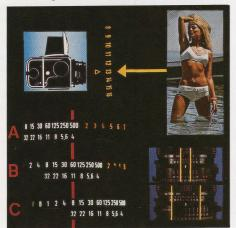
With the lens set to EV, you can select the aperture that provides the desired depth of field. The shutter speed that exposes the image correctly is automatically set. As an example, at EV13 an aperture of f/4 automatically sets the shutter speed to 1/500 second (A). If you decide to go to f/11, the shutter speed automatically moves to 1/60 second (B), or to 1/8 second at f/32 (C).
