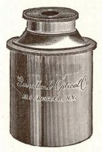
This lens is an achromatic combination of novel construction consisting of a double convex crown glass lens and a negative miniscus flint glass lens, cemented together and mounted in brass with adjustment to focus. The lens is perfectly aplanatic.
