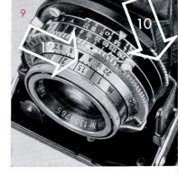
accurate focus are vertical lines, such as the edge of a house, a tree, etc.) (ill. 8). As soon as the contours coincide the lens is accurately focused at the correct distance required. Moreover, the correct distance may be read off from the black distance setting mark on the scale (12) of the lens ring (ill. 9).
