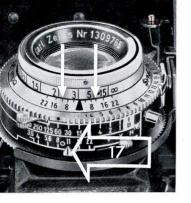
(13). Diaphragm figures will be found on the right and left side of the distance setting mark. The figures on the distance scale (12) opposite these stop figures indicate the extent of the depth of field. The strokes without figures beside the triangular mark indicate the depth of field at stop f: 4
