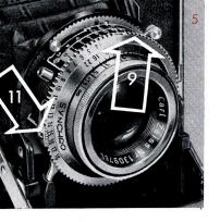
Since this lever has a limited travelling space only, the exposure value can sometimes only be set by also turning the adjusting ring (9) on which the exposure value scale is placed. When the correct exposure value has been set
