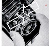
"B") is indicated the exposure time required is 2 seconds. If it is intended to use a smaller stop (to do this pull out lever (11) as it is done for the setting of the exposure value), the exposure time required can be read off from the exposure meter as described on page 10. This means, of course, that the exposure value setting is out of action. When the shutter setting is changed from "B" to one of the various shutter speeds, the exposure value must also be re-set in the first place.
