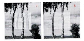
outlines of the object will appear double (ill. 7). By turning the milled ring (10) with the middle finger of the left hand these double outlines in the centre of the measuring field can be brought to coincidence. (The best objects for obtaining an
