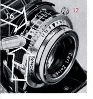
speed does not exceed  $1-\frac{1}{30}$  second. However, it must be borne in mind, that the flash duration of most bulbs is appr.  $\frac{1}{100}$  second so that you actually expose  $\frac{1}{60}$  to  $\frac{1}{100}$  second. Electronic flashes *must* always be fired with the "X" setting. *The "M" setting* allows for
