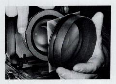
Filters can be rapidly exchanged without screwing or locking. In spite of this, they are held in place reliably, perfectly flat, free from strain and with maximum care. The specially designed glare shield positively avoids vignetting even when full use is made of camera movements.
