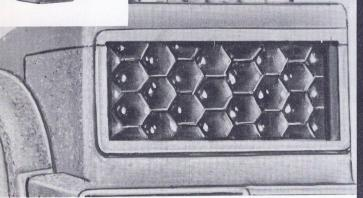
THE ELECTRIC EYE instantly measures the intensity of light and adjusts the lens aperture for correct exposure of the film, as soon as the operating lever is pressed.
