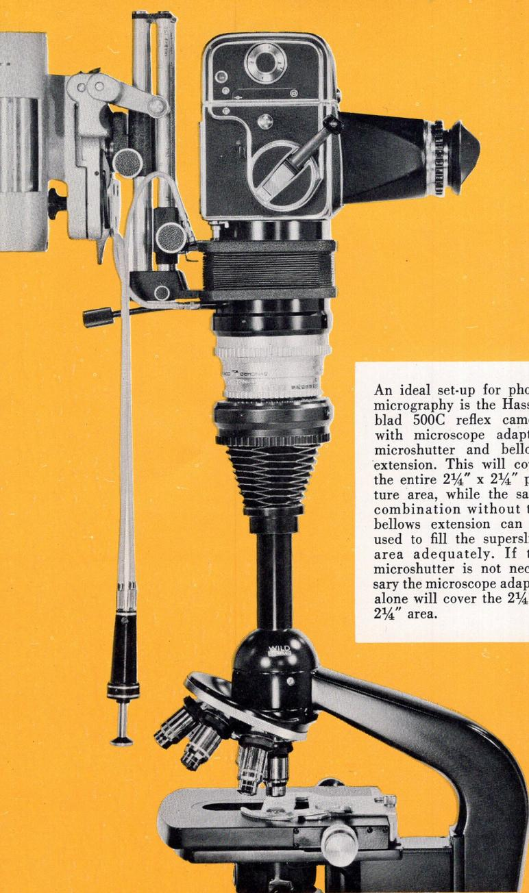
An ideal set-up for photomicrography is the Hasselblad 500C reflex camera with microscope adapter, microshutter and bellows extension. This will cover the entire  $2\frac{1}{4}'' \times 2\frac{1}{4}''$  picture area, while the same combination without the bellows extension can be used to fill the superslide area adequately. If the microshutter is not necessary the microscope adapter alone will cover the  $2\frac{1}{4}'' \times 2\frac{1}{4}''$  area.
