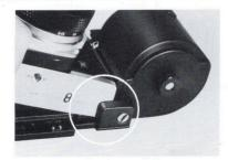
4) Place the left side of the camera (side with Rewind Crank) on the Camera Stage of the Film Back and push the camera towards the Back until the two units are flush against each other.
