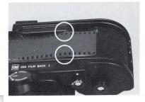
6) Make sure the film is evenly spaced between the film guides and that the perforations of the film engage with the Exposure Counter Sprocket.
