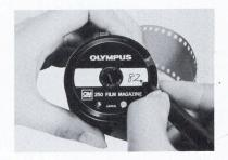
4) To remove the right magazine, pull down on the Fork Knob of the right chamber and remove the magazine by inverting the Film Back and shaking gently.
