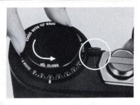
9) Turn the Open/Close Knob on top of the left chamber to "CLOSE". This extends the Camera Holder and opens the Supply Magazine.
