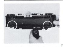
3) Place the supply magazine in the left chamber and the take-up magazine in the right. Line up the red index marks on the magazines with the white index marks on each chamber and snap the magazines into place.
