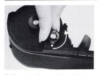
3) Turn the Camera Clamp Knob at the base of the right Magazine Chamber in the opposite direction of the arrow until it stops. This will release the Camera Clamp Plate and allow you to attach the Film Back to the OM-1.
