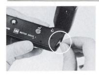
6) Attach the Motor Drive 1 to the camera. Open the Coupling Gear Cover on the base of the Motor Drive 1. The gears must be completely exposed to ensure proper coupling with the Film Back.
