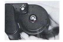
7) Make sure the units are attached properly by operating the camera's film advance lever or the motor drive. The Fork Knob at the base of the right Magazine Chamber will rotate indicating that the film advance mechanism is functioning.
