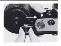
5) While pressing the right side of the camera against the Film Back, turn the Camera Clamp Knob in the direction of the arrow until it stops. The Camera Clamp Plate will close locking the camera firmly against the Film Back 1.
