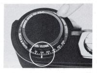
12) Set the Film Type Indicator on the top of the left chamber as a reminder of the type of film you are using. (Make sure the Open/Close Knob has not been moved from the "CLOSE" position.)
