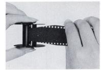
2) Cut and taper the end of the bulk film to make a leader. Hold one of the spools in one hand and with the film in your other hand, insert the film leader into the spool's slot, emulsion side (dull side) down. Do not fold back the leader.
