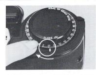
1) When the motor drive stops and the Exposure Counter indicates the last frame has been exposed ("0"), turn the Exposure Counter back to 10 frames ("10"). Cover the camera lens and advance the film 6 frames. This will safely wind the last few exposed frames into the take-up magazine to prevent fogging when opening the back.
