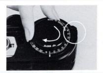
8) Turn the Open/Close Knob on the right chamber to "CLOSE". This locks the Camera Clamp Knob and Rear Cover Lock Key into place, and opens the Take-up Magazine.
