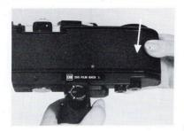
7) Place the rear cover of the 250 Film Back on by hooking the left end onto the catch provided at the left end of the Back. Carefully press the right end into place so the hooks of the cover slide under the edge of the back and snap into place.
