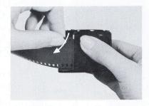
3) Remove the left film magazine, and cut the film by pressing it against the film cutter of the take-up magazine and tearing towards you and down. This leaves a leader extending from the left magazine to be used for spooling the remaining unexposed film.
