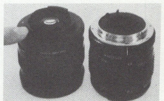
Yashica bayonet (right) features solid stainless mount while Contax (left) opts for a screw-on flange. Yashica used the latter mount on the 38-90mm zoom.
