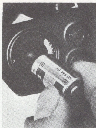
Six-volt silver oxide battery resides in compartment underneath camera.
