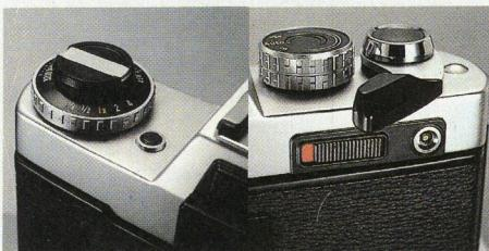
*Exposure Compensation Dial for Correcting Backlit or Spotlighted subjects. Lockable Exposure Check Button for Special Exposure Reading.*
