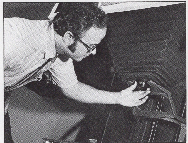
The heart of a vertical process camera is the lens. Many vertical cameras use Goerz lenses as standard equipment. Photo Courtesy Kenro Corporation.
