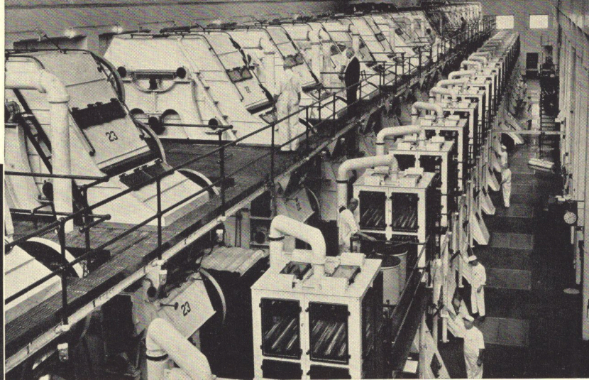
Converting fluid "dope" into endless sheets of the familiar transparent film base, . . . which is very nearly invisible as it passes over the polished rollers
