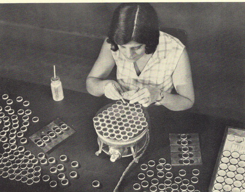
Use of two glasses in one lens element corrects certain optical aberrations; so "crown" and "flint" types are cemented together
