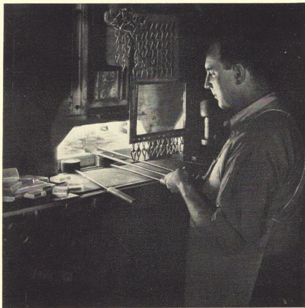
The first step: optical glass is softened in a furnace with 1600 degrees of temperature, and then it is molded into lens discs
