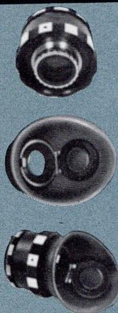
**AUTOMATIC CLOSURE EYEPIECE** This special eyepiece features an automatic closure mechanism that is a welcome convenience and safeguard. The eyepiece mechanism opens and closes automatically when eye pressure is applied or released. A manual over-ride is provided to keep the eyepiece open if so desired. The automatic closure eyepiece is available as an accessory, or as an optional extra. It may be used on the Arriflex 35 2C as well as on all late model Arriflex 16 cameras.
