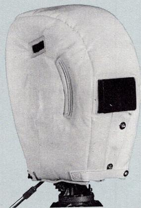
**SOUND BARNEY** This multi-layered camera covering, has excellent acoustical characteristics and it can dampen sound as much as 60%. For tough location jobs, where standard sound blimps cannot be used, the Barney can help to bring back good synchronous sound. The Barney also serves to protect the camera against the weather. Heater Barneys, to operate on 115 volt, AC, are also available. Made in U.S.A.
