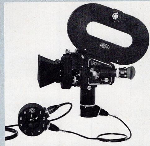
**Arriflex 35 Model 2CBHS,** with all the features of the Model 2C, plus special 32 volt, DC motor, separate speed-control rheostat, and special tachometer, for operation to 80 fps.
