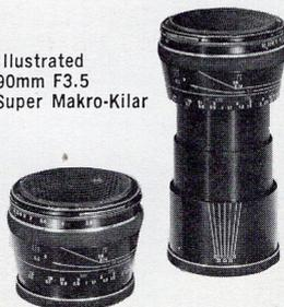
**MACRO LENSES** Makro - Kilar lenses (40mm F2.8 and 90mm F3.5) are ideal for extreme close-ups. They focus from infinity to 4" and 5" respectively, providing image ratios right down into the 1:1 range without extension tubes or bellows attachments. These remarkable lenses plus Arriflex's famed thru-the-lens reflex viewing system makes difficult macro shots exceptionally easy and economical.
