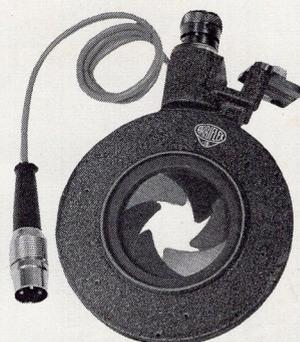
**AUXILIARY SHUTTER** — The Auxiliary Shutter serves as a capping shutter in single frame filming. Its purpose is to prevent fogging in single frame filming, where light levels are high and a frame of film remains in the camera gate for a relatively long time. The Auxiliary Shutter operates on its own 24 volt DC solenoid and may be automatically controlled by the Arriflex Single Frame Motor.
