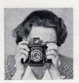
The camera rests firmly in the palms of the hands. Shutter is released in this position the forefinger of the right hand can operate the shutter release.
