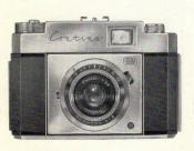
The Contina I is the "economy" model lacking the built-in photoelectric exposure meter of models II and III. It incorporates the same quality, finish and ruggedness which characterize the other models, and is ideal as a "second" camera. Fitted with Pantar f/2.8, 45 mm lens in Prontor SVS shutter with speeds to 1/300th second.
