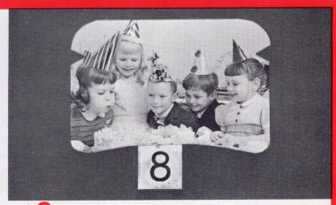
**EXPOSURE SCALE,** visible in viewfinder, shows exposure value of scene being shot. Black flag indicates when light is insufficient for good movies.
