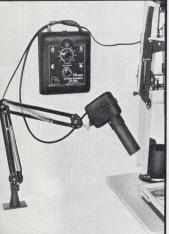
Photocell-controlled enlarging exposure timer. Dial proper setting, aim photocell, push "Exposure" button, and Timega turns off enlarger when paper is properly exposed. Provides uniform print quality even for varying density negatives. Builtin dial safelight.
