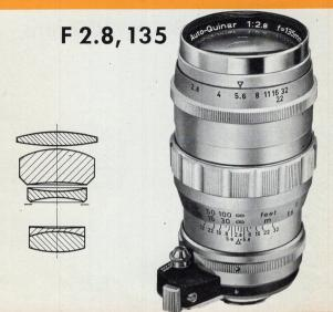
The f/2.8, 135 mm Auto-Quinar Telephoto lens with instant-reopen automatic diaphragm is a fast telephoto lens of superior design. Comprised of a 5-element lens system, this lens meets the highest standards for color, sharpness and performance. There are 8 diaphragm stops from f/2.8 to f/32. Angle of view is 18°. Lens focuses from infinity down to 5 feet, and can be operated both automatically and manually. Leather case and sunshade furnished with lens at no addiprice
