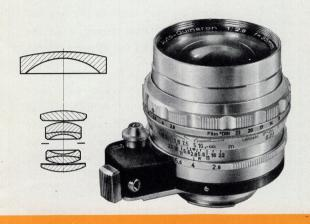
The renowned 7-element f/2.8 Auto-Quinaron 35 mm Wide Angle lens has an instant-reopen automatic diaphragm. It focuses from infinity down to  $4^{1/2}$  inches from the front element of the lens to the subject. Does not require bellows extensions or extension tubes for closeups. The angle of view is  $62^{0}$ , smallest of 7 diaphragm stops is f/22. Lens can also be operated manually if desired.
