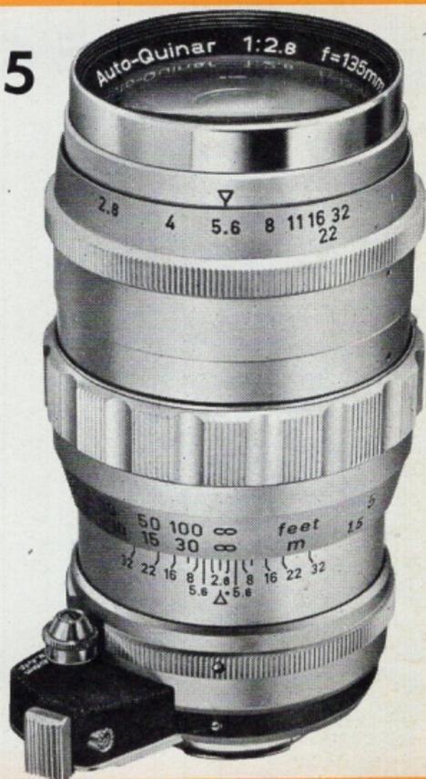
The f/2.8, 135 mm Auto-Quinar Telephoto lens with instant-reopen automatic diaphragm is a fast telephoto lens of superior design. Comprised of a 5-element lens system, this lens meets the highest standards for color, sharpness and performance. There are 8 diaphragm stops from f/2.8 to f/32. Angle of view is  $18^{\circ}$ . Lens focuses from infinity down to 5 feet, and can be operated both automatically and manually. Leather case and sunshade furnished with lens at no additional charge.
