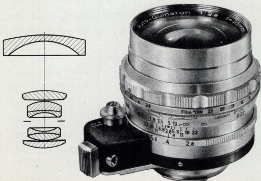
The renowned 7-element  $f/2.8$  Auto-Quinaron 35 mm Wide Angle lens has an instant-reopen automatic diaphragm. It focuses from infinity down to  $4\frac{1}{2}$  inches from the front element of the lens to the subject. Does not require bellows extensions or extension tubes for closeups. The angle of view is  $62^\circ$ , smallest of 7 diaphragm stops is  $f/22$ . Lens can also be operated manually if desired.
