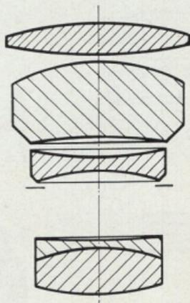
The f/2.8, 135 mm Quinar Telephoto lens has a preset diaphragm. It renders a 2.7 time magnification over a normal lens, and is an ideal lens for sports, bird, nature and candid photography.
