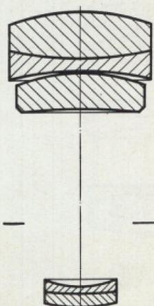
The  $f/4.5$ , 200 mm Steinheil Tele-Quinar is a true telephoto lens with preset diaphragm. It has a 5-element lens system and renders a 4-time magnification in comparison to a normal 50 mm. lens. The Tele-Quinar is corrected according to the latest scientific standards, and is highly recommended for color. There are 7 diaphragm stops to  $f/32$ ; lens focuses down to 7 feet. Angle of view is  $12^\circ$ . Leather case and sunshade are furnished at no additional charge.
