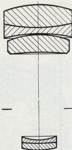
The f/4.5, 300 mm Tele-Quinar with preset diaphragm is an extraordinary telephoto lens. It has a 5 element lens system with an  $8^{\circ}$  angle of view. The lens is corrected to a high degree, making it a 'preferred' lens for color photography. For outdoor shots, nature, bird, sports, and marine work, the lens will perform with outstanding results. Diaphragm closes down to f/32. Finished in ebony and chrome mount.
