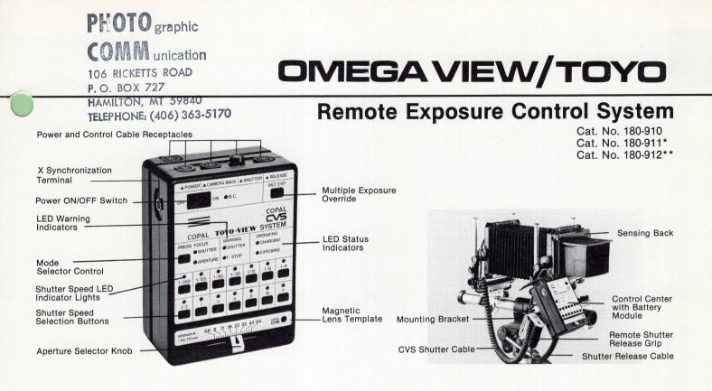
The Omega View/Toyo Remote Exposure Control is a programmable exposure system designed by Copal (CVS) that permits many Omega View/Toyo large-format users to set all aperture and shutter information remotely and precisely. The photographer never has to step from behind the camera to adjust exposure settings; especially important when operating a view camera at an extended height.
