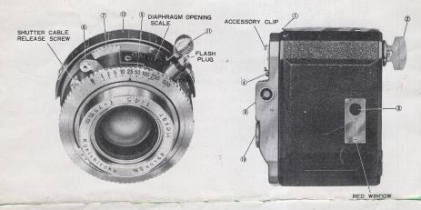
Loading: Be sure that the shutter is closed, open the camera back by sliding the back catch (1), and place the film in empty chamber. Break the gummed strip and slide the leading paper across the film truck. Insert in the slit of the take-up spool and wind a few turn by the winding key (2), Close and lock the camera back and turn the winding key until the figure "1" appears in the red window (3).
