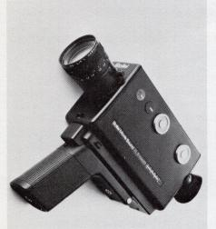
The Rollei SM8XL super 8 sound movie camera (page 7) is ideal for your most discerning Super 8 customers. The SM8XL features an 8 element f/1.4 Schneider Variogon zoom lens, 7mm to 56mm (8:1) with macro focusing. The combination of a  $235^{\circ}$  low light shutter and the f/1.4 lens are ideal for indoor on-location available light filming. Hi-fi quality sound components, Bogen sound heads and Siemens electronics, are used for superior quality sound reproduction.
