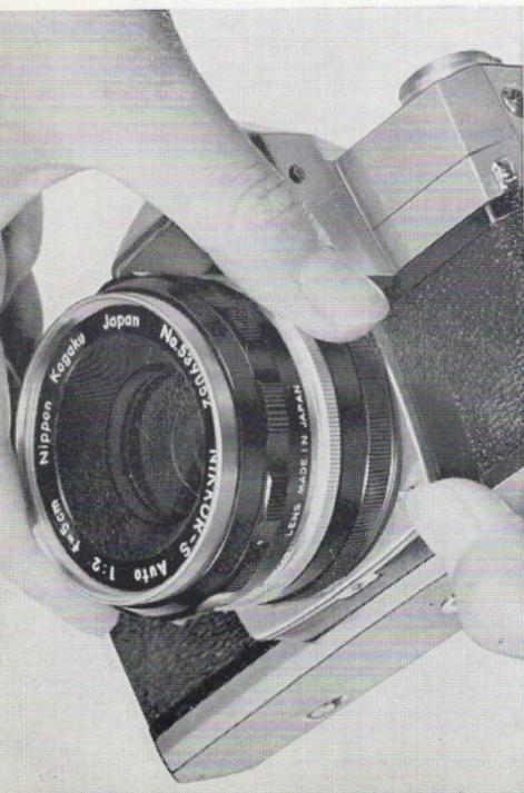
To remove the lens, hold the camera as shown left, depress the lock button found underneath the lens and turn the lens barrel clockwise until the black indicator dot on the milled ring of the lens lines up with the black dot on the camera body as shown above.
