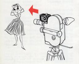
The very narrow acceptance angle of the Bolex exposure meter makes it especially suitable for this method of measurement. In fact, this method should be used in the majority of cases.
