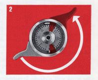
cates the actual number of exposures on your film. Note that the rewind crank rotates of its own accord in the opposite direction to that indicated by the arrow: this allows you to check that the film is being advanced correctly.
