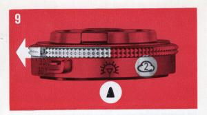
tically to the sun symbol when it is released. The figure 2 within the cloud symbol indicates that the dull weather corrector corresponds to a filter-factor correction of 2x, and it may also be used for this purpose. If the aperture requires less than one full f/stop correction, then the ring need only be turned by a correspondingly smaller amount.
