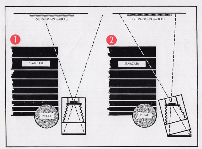
Quite often, an oblique camera position is unavoidable due to architectural structures, such as posts, pillars or staircases interfering with the viewpoint. Again the swing back is adjusted horizontally so as to be parallel to the front of the subject. Sharp focus is provided by swinging the lens into parallel position to the film plane.
