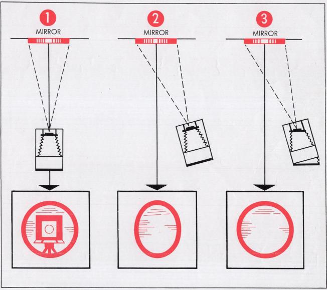
It sometimes happens that a subject must be photographed without its front surface being at right angles to the camera axis. The reason for this may be a strongly reflecting surface of the subject, or lack of space. In both cases, the camera must be placed slightly to one side, thus producing a distorted image of the subject. As a result, the picture looses its front view appearance.
