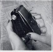
Replace the back, making sure the lock is secure to avoid accidental fogging of the film.
