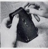
Wind the film until the figure 1 appears in the center of the green window on the back of the camera.
