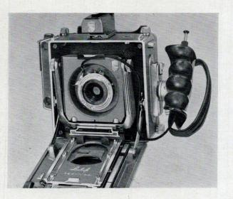
FOR USE WITH 90 mm WIDE-ANGLE LENS. After Inserting 90 mm cam (see above) pull out lens standard to (black) infinity stops; drop bed to second notches of strute by pushing down on struts — as if to close camera — and letting down bed. Dropping the bed prevents
