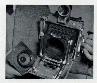
INTERCHANGE OF LENSES is a matter of seconds. Pull out lens standard half-way on upper track; raise locking bar (27) and lift lens with lens board up and out from retaining brackets (30). To insert lens, seat lower edge of lens board on brackets; press upper edge of lens board against locking bar until it snaps into position.
