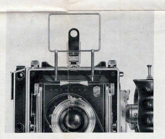
THE WIRE FRAME FINDER is recommended especially for action shots. It is inserted in the socket (25) atop the lens board frame; the peep-sight is slid into the special mounting shoe on the camera body, and folded up. Parallax correction is provided by raising the peep-sight and refering to the parallax scale. For vertical shots
