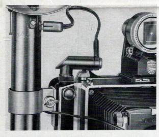
THE KALART FOCUSPOT ATTACHMENT is used for focusing in the dark with the Multifocus Rangefinder at close and middle distances. The Focuspot is attached to the rangefinder housing after removal of the milled dust cover (6), and connected to a flash unit provided with 4 or 6 Volt outlet. For correct focus the two light spots projected on the subject through the rangefinder are brought into coincidence by turning the focusing knob (18) of the Super Technika.
