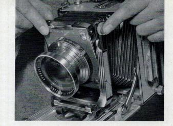
FRONT TILT THROUGH HORIZONTAL LENS AXIS. Loosen locking knob (28). When the opposite release knob (26) is pressed in, the lens board frame may be tilted forward or backward to a maximum of 15° in either direction, and fixed at Click stop for zero position. ny angle by tightening knob (28).
