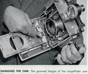
CHANGING THE CAM. The grooved tongue of the rangefinder cam (13) permits easy, one-hand insertion of the cam into the cam shoe (31). With the upper track racked forward (as shown above) the cam is lifted slightly, and pulled out by the right hand; when cam is inserted, slide it into the slice as far as it will go to stop. (The Super Technika IV may be closed when no cam is in the shoe).
