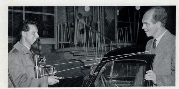
Rangefinder focusing with the Kalart Focuspot and viewing can be carried out separately or together whereby the viewfinder becomes a combined range-viewfinder by observing the merging of the two light beams projected by the Focuspot in the viewfinder image.
