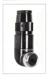
Used directly on the eyepiece frame of the Super D and Super DM cameras and via eyepiece adapter on the UNI, Unirex and IC-1 cameras. Used for viewing and focusing at right angle to the optical exis, with 1x magnification, and may be revolved 90° or full 360° as desired.
