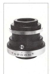
Three ring set for connecting the camera body to the telescope in astrophotography. Can be connected to telescopes with drawtubes of 30.2 mm and 36.2 mm outer diameters or with the T mount adapter.
