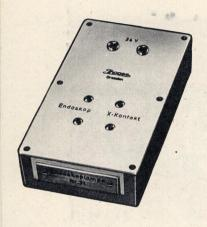
of exposure. The Overrunning Switch Apparatus is designed for use in conjunction with the EXAKTA VX IIa and IIb to effect this switchover automatically; it is connected to the X-contact of the camera. A 24 V source of current is required, whilst a 12 V tungsten lamp is fitted in the endoscope. During the preparatory stages the lamp is run on an 8 volts supply only, whilst during the exposure the voltage is raised momentarily to 24 V without giving it time to damage the lamp.
