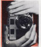
the left hand, while the index finger of the right hand, resting lightly on the exposure counter (16), is used to press the shutter release button.
