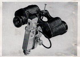
One ocular of the binoculars used in conjunction with the camera serves to take the picture, whilst the other one is used as the viewfinder, for sharp focusing and for the observation of the subject. The camera focusing disc should be set always at ∞ (infinity). The following instructions describe separately the use of the Minox camera in connection with binoculars with and without central screw focusing wheel.
