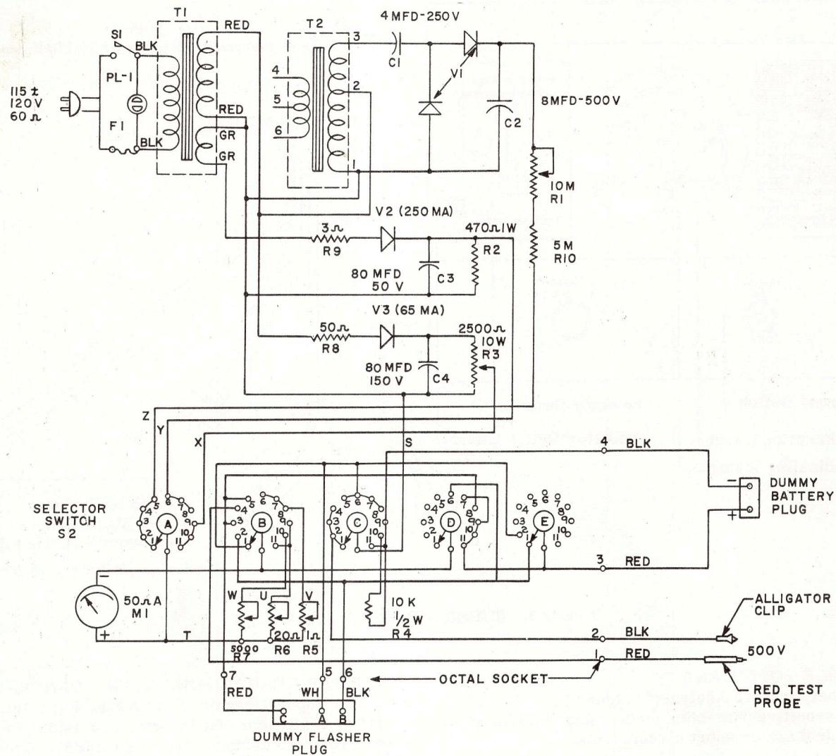
Figure 3A. SUPER GRAPHIC ANALYZER - SCHEMATIC DIAGRAM
