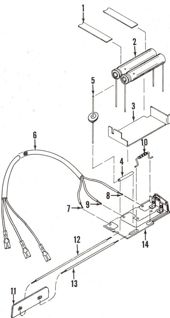
Figure 5A. CIRCUIT PLATE COMPLETE
