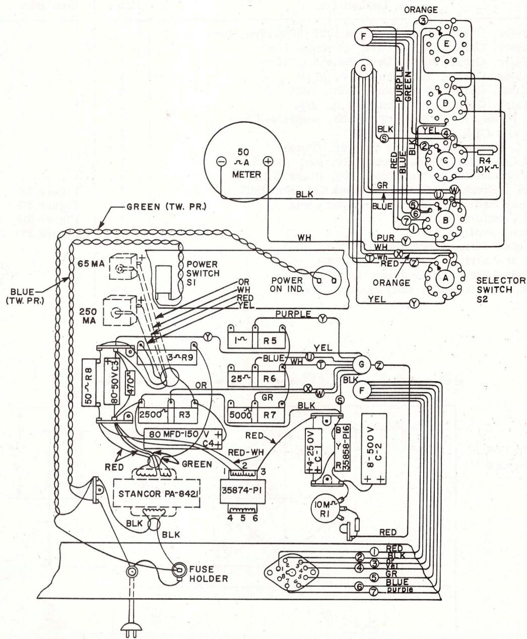
Figure 3B. SUPER GRAPHIC ANALYZER - WIRING DIAGRAM
