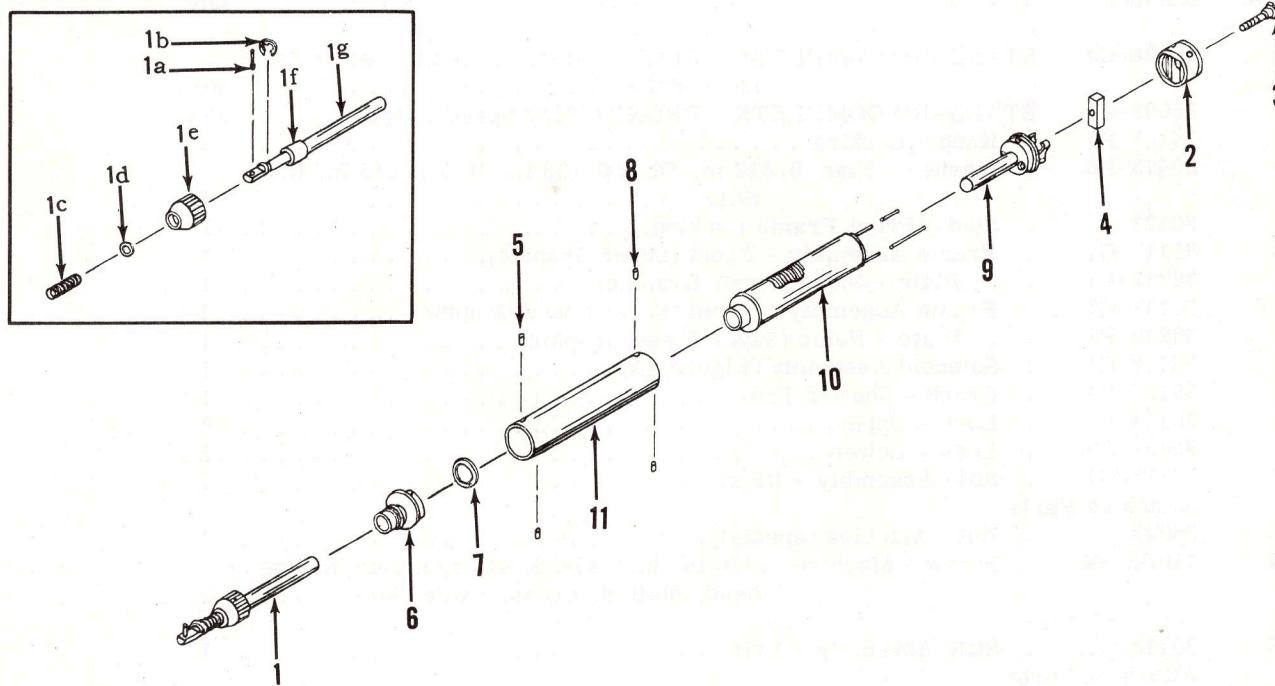
Figure 4A. SOLENOID ASSEMBLY
