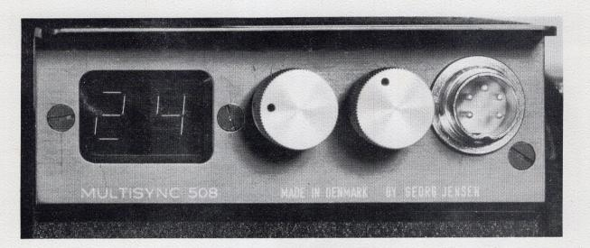
igencies of the individual camera design dictate certain variations: e.g., instead of an over-ride button for out-of-crystal-sync recovery, the operator has a control knob to restore pre-modification operation.
