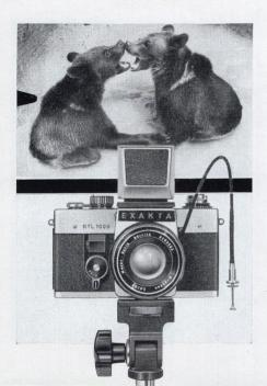
2. The image in any of the viewfinder systems (Finder Hood, Penta Prism, and TTL Penta Prism) will be visible even after the shutter has been released (instant return mirror). The red warning signal in the image in the viewfinder system indicates that the camera is not yet ready for action, and that the rapid-wind lever (9) must be cocked before the shutter is ready for release (See illustration: image seen through the Penta Prism).
