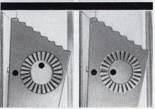
Swing the release lock (4) to the stop on the right (marking dots are staggered): the shutter can be released by pressing on the right-hand release (5). When you have finished taking pictures, swing the release lock (4) to the stop on the left (the marking dots are opposite each other): now it will be impossible to release the shutter, which means protection against unintentional exposures. (No locking in case of the left-hand release (16).)
