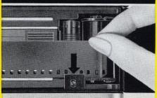
3. Pull the beginning of the film (29) as far as the green mark (35), and push it with its (lower) perforation from above under the film rest (33) and, accordingly, over the film-wind sprocket (32). The catch bow of the take-up spool (34) must not stand upwards!
