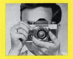
and index finger of the left hand, the right index finger being used for releasing the shutter.
