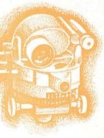
Army and Navy guns, in many sizes, are sighted or aimed by one or more of many Kodak-made optical instruments for fire control—such as the intricate aiming circle, above.
