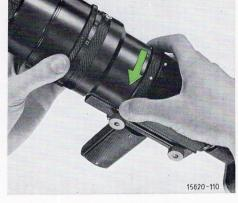
Turn the bayonet locking ring (5) until its red dot is aligned with the red dot on the mount. Insert the aperture tube (6) by pressing straight in so that its red dot lines up with the other two, as shown above. Finally, lock the aperture tube in position by turning the locking ring (5) to the left, as far as it will go. Note that in the locked position, the red dot on the locking ring finds itself at the left-hand center of the rapid focusing mount.
