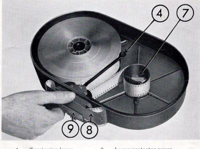
4 = Tensioning lever8 = Loope protector cover7 = Take-up core9 = Retaining piece for 8
