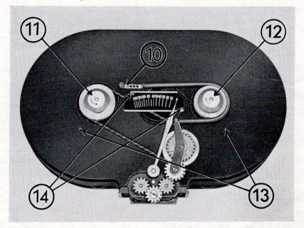
10 = Four-hole spring loaded eyelet
