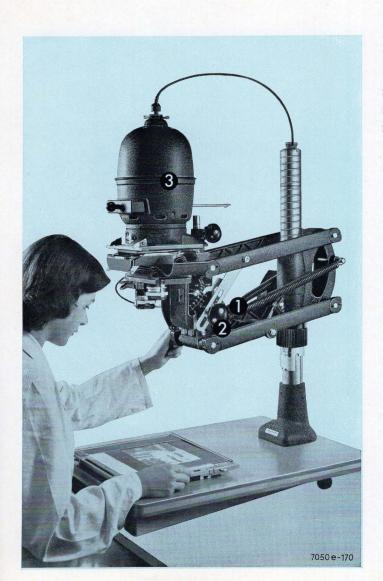
The head of the FOCOMAT II c is raised and lowered smoothly and easily by means of parallelogram arms with particularly well-placed non-torque levers and counterbalancing springs ①. A conveniently located clamping knob ② locks the enlarging head at any desired height within its operating range. A large rubber stop softens impact at the lower end position.
