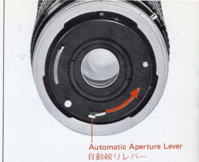
checked as follows. Remove the lens from the camera. To unlock the Breech-Lock Mount Ring, press the Mount Lock Pin located above the Positioning Pin with a pointed object, such as a pencil, and rotate the Breech-Lock Ring until it stops. While looking through the lens after setting the aperture ring at f/5.6 or f/8, push the automatic aperture lever to check the diaphragm movement.
