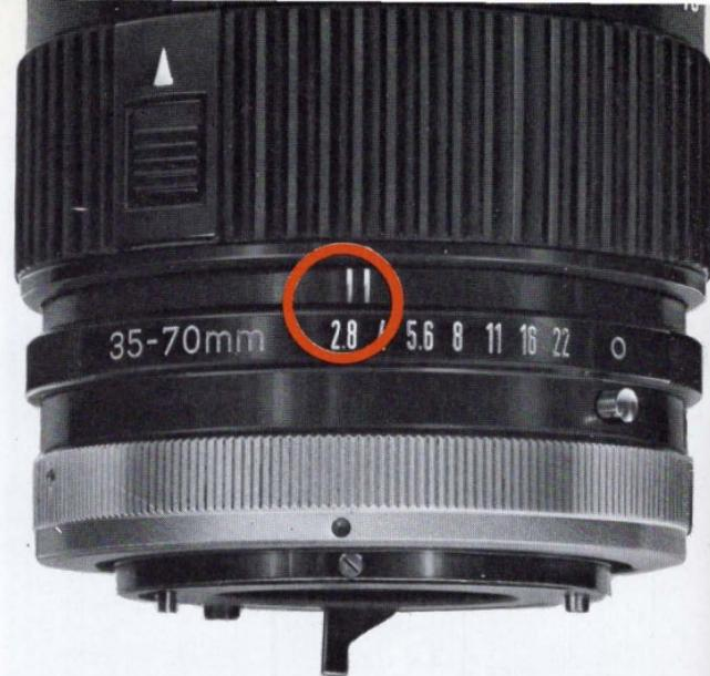
There are two aperture index marks; the blue mark is for 35mm, and the pink one for 70mm. For 50mm, the value should be read between the two indicators.
