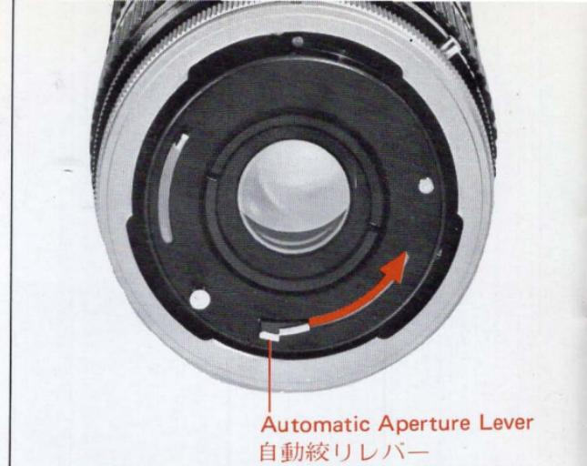
checked as follows. Remove the lens from the camera. To unlock the Breech-Lock Mount Ring, press the Mount Lock Pin located above the Positioning Pin with a pointed object, such as a pencil, and rotate the Breech-Lock Ring until it stops. While looking through the lens after setting the aperture ring at f/5.6 or f/8, push the automatic aperture lever to check the diaphragm movement.
