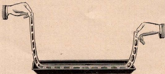
Fig. 15.—DRAWING FILM THROUGH DEVELOPER.
