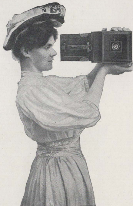
Showing Auto Graflex used as a deceptive angle camera
