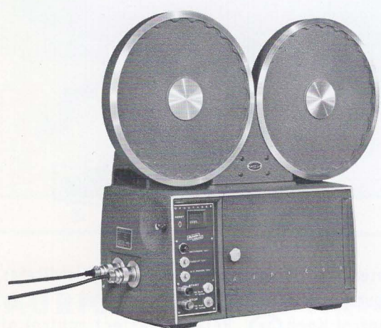
16mm "AURICON-1200" RECORDER Model RM-30... 1200 ft. film capacity for up to 33 minutes of continuous recording, reversible synchronous-motor driven for "A" or "B" wind "Double-System" 16mm Optical Sound-On-Film operation. Available for Variable-Area or Variable-Density Recording.
