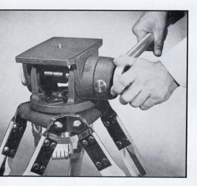
22 inch pan-tilt handle can be adjusted to exact angle for most comfortable position and accurate control of camera movement. Interlocking precision-machined teeth provide rigid positioning of handle.
