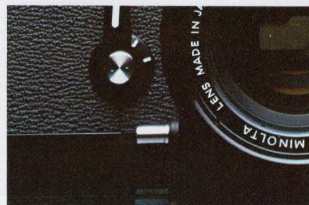
Preview button on electronic Minolta XE-7 (shown) and other Minolta 35mm SLR's permits stopping lens down to taking aperture for judging depth of field visually on viewing screen.
