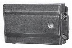
black paper on the film spool is passed over the face of the carrier to the receiving spool. A retarding ratchet is provided whereby the film may be drawn absolutely flat after it is in position for exposure, affording a true recording plane. The Graflex Roll Holder is fitted with a dark slide, which permits the removal of the Holder from the camera before the entire roll has been exposed, without injuring the film.
